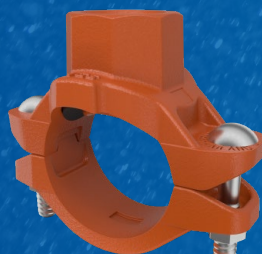
VG122 Threaded Mechanical Tee 1¼ x ½ to 6 x 2½ NPS
